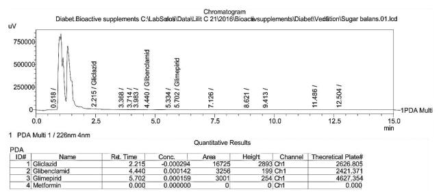
Figure 4. "Dialevel" sample injection chromatogram.
