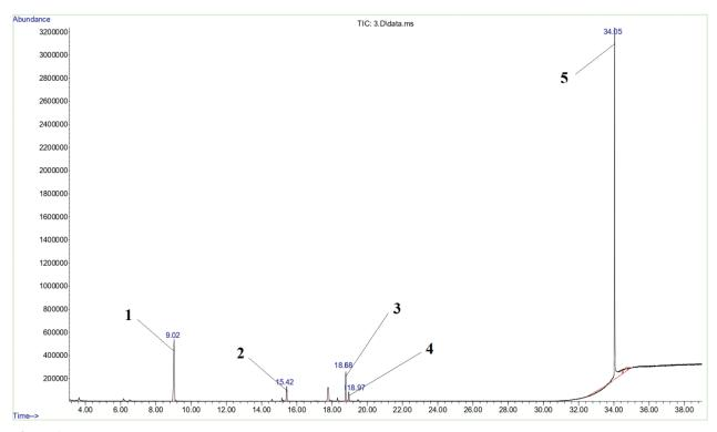
**Figure 2.** GC-MS chromatogram of free carbohydrates in *Taraxacum officinale* roots (1 – *D*-arabinose, internal standard; 2 – *D*-glucose; 3, 4 – *D*-fructose; 5 – sucrose).
