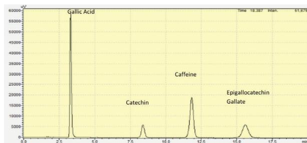
**Figure 1.** HPLC Chromatogram separation of EGCG, caffeine, and catechin (10 µg/mL) using mobile phase methanol-ortho phosphate-water (20:0.1:79.9 v/v/v) with flow rate 1 mL/min delivered isocratically and UV detected at  $\lambda$  280 nm.
