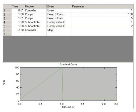
Figure 2. Gradient curve.
