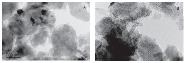
Figure 1. TEM images of empty (picture A) and indomethacin-loaded (picture B) particles.
