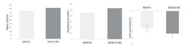
**Figure 2.** DLS determination of main physicochemical characteristics (size, polydispersity index and zeta-potential) of empty (MCM-41) and indomethacin-loaded particles (MCM-41 IND).
