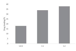
**Figure 5.** Drug loading rate (%) with using of different MCM-41/indomethacin ratios in the incubation stage.
