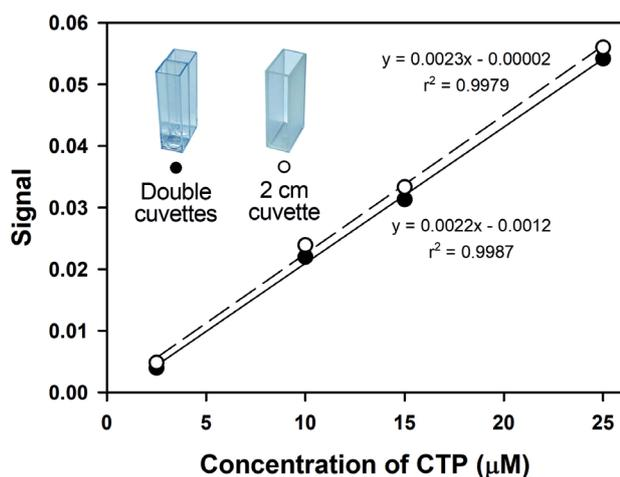
**Figure 7.** Standard curves obtained from signal acquisition using double 1-cm pathlength cuvettes and a 2-cm pathlength cuvette.
