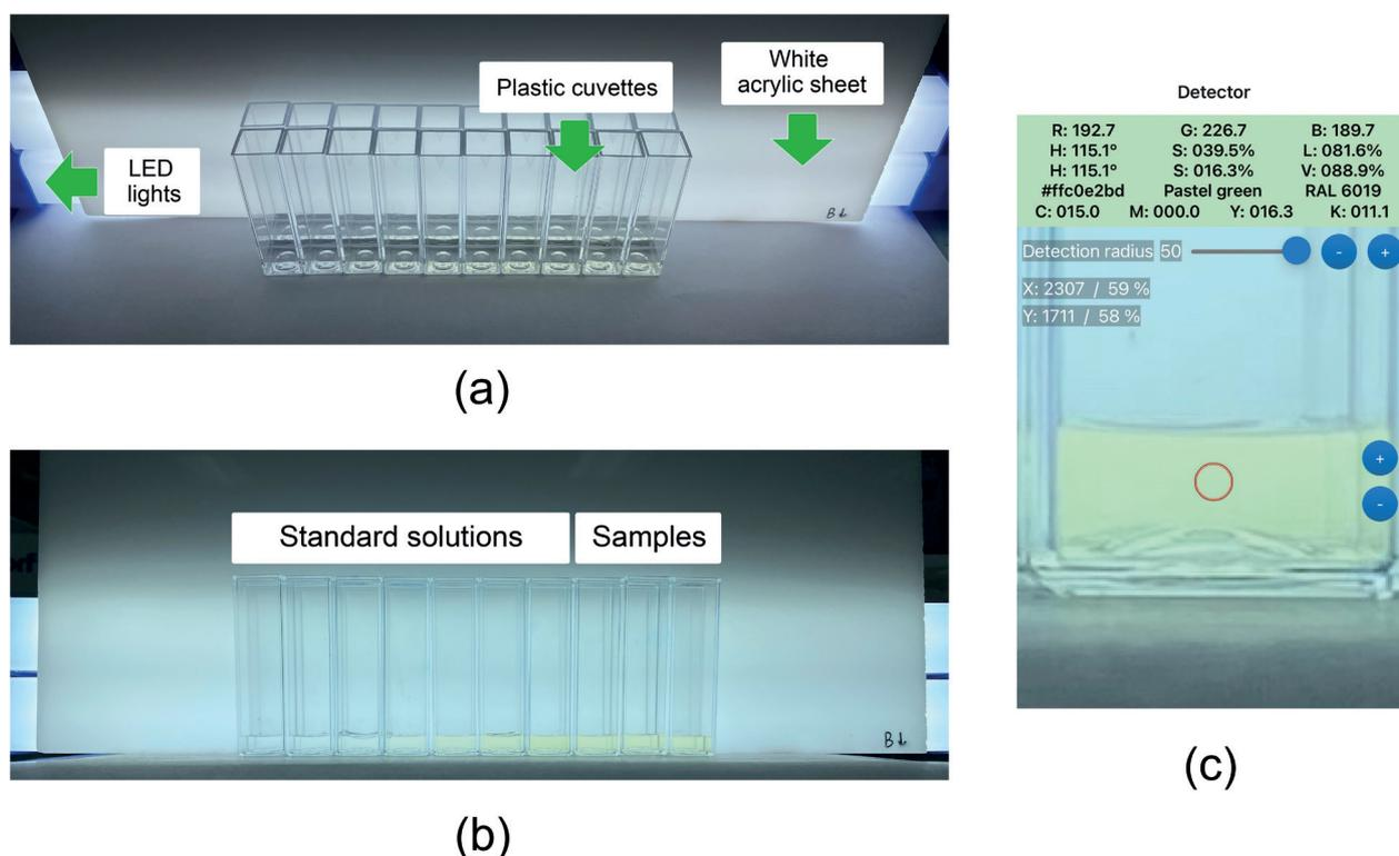
**Figure 1.** Alignment of cuvettes for photography from top view (a) and front view (b), and measurement of RGB colors on the digital image using the RGB Color Detector application (c).
