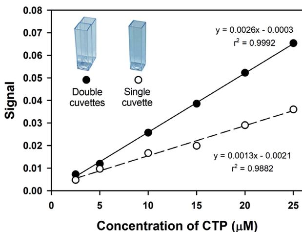
**Figure 4.** Standard curves obtained from signal acquisition using a single cuvette and double cuvettes.
