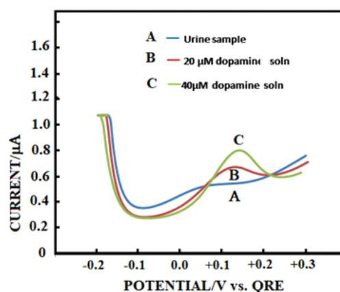
**Figure 6.** Differential pulse voltammograms for an iodine coated electrode in 0.1 M PBS (pH 7) of spiked with (A) spiked with urine sample only (B) spiked with 20 μl of dopamine (C) spike with 40 μl of dopamine. Scan rate = 5 mV s<sup>-1</sup>, modulation amplitude = 50 mV, pulse repeat time = 1 s.
