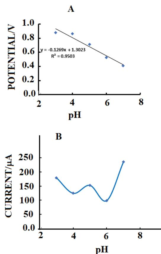
**Figure 2.** The effect of pH on (A) anodic peak potential and (B) anodic peak current. Anodic peak potentials and currents were extracted from cyclic voltammograms of iodine-coated platinum electrode in 0.1 M PBS solution containing 1.0 mM dopamine at different pH values.  $dE/dt = 100$  mV/s.
