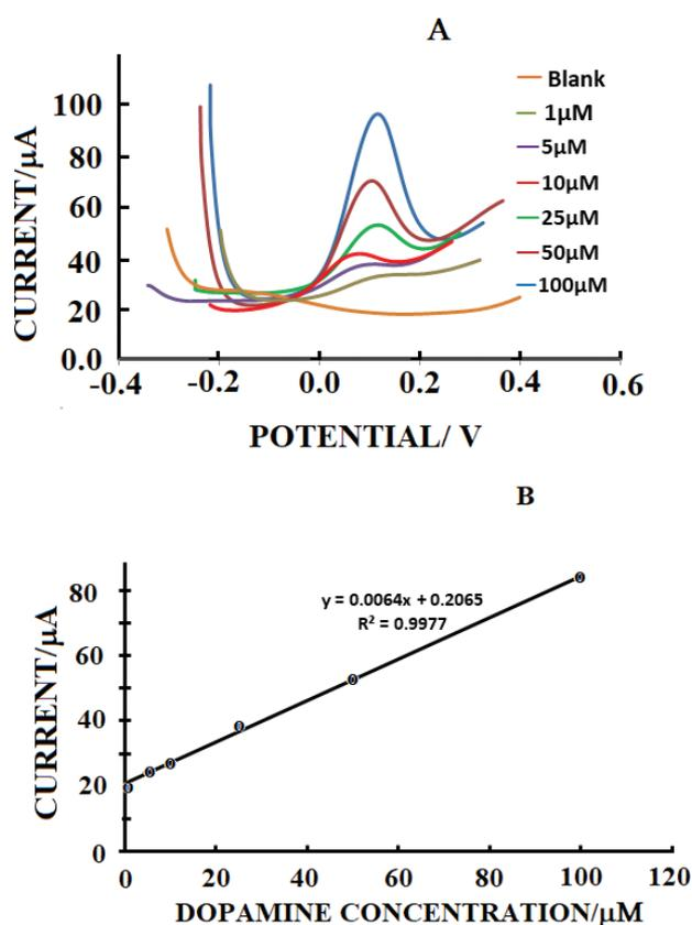
**Figure 4.** **A.** Differential pulse voltammograms of an iodine-coated platinum electrode in 0.1 M PBS (pH 7) containing different concentrations of dopamine. scan rate:  $5 \text{ mV s}^{-1}$ , modulation amplitude = 50 mV. pulse repeat time: 1 s. **B.** A plot of the concentration of dopamine vs. the peak currents extracted from the corresponding voltammograms (in Fig. 4A).
