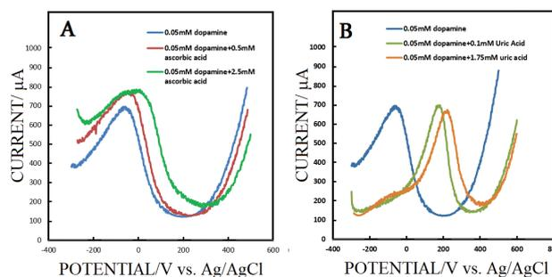
**Figure 5.** A. Differential pulse voltammograms for the iodine coated electrode in PBS containing (A) (blue) 0.05 mM dopamine, (red) 0.05 mM dopamine + 0.5 mM ascorbic acid, and (green) 0.05 mM dopamine + 2.5 mM ascorbic acid. B. (blue) 0.05 mM dopamine, (green) 0.05 mM dopamine + 0.1 mM uric acid and (orange) 0.05 mM dopamine + 1.75 mM uric acid.
