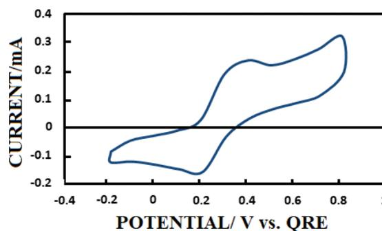
**Figure 1.** Cyclic voltammogram of an iodine-coated platinum electrode in 0.1 M PBS solution containing 1.0 mM dopamine. Experimental conditions:  $dE/dt = 100$  mV/s, pH = 7. This anodic peak was considered for quantification of dopamine in urine and serum samples.
