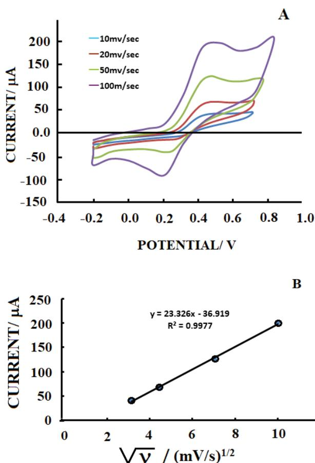
**Figure 3.** The effect of scan rate on the anodic peak current for oxidation of dopamine at iodine-coated platinum electrode. **A.** Cyclic voltammograms of dopamine electrooxidation at iodine-coated electrode in 0.1 M PBS (pH 7) solution containing 1.00 mM dopamine. Scan rate = 100 mV/s **B.** A plot of anodic peak current vs.  $(\text{scan Rate})^{1/2}$ , where  $n$  is the scan rate of the recorded voltammograms in (A).
